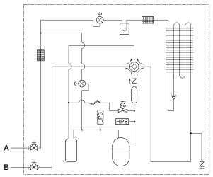
+V+Service port (with 5/16" flare) 本 Stop valve Filter Check valve Muffler Solenoid valve PCB cooling Capillary tube Electronic expansion valve 4-way valve High pressure switch
