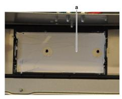
a Thermal interface grease on heat sink
