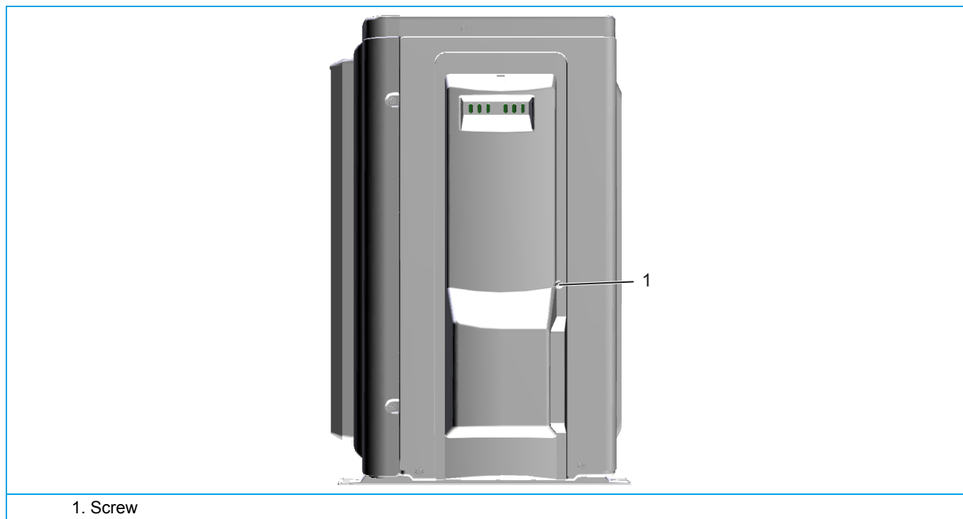
Figure 3-11: Removing refrigerant connection cover
