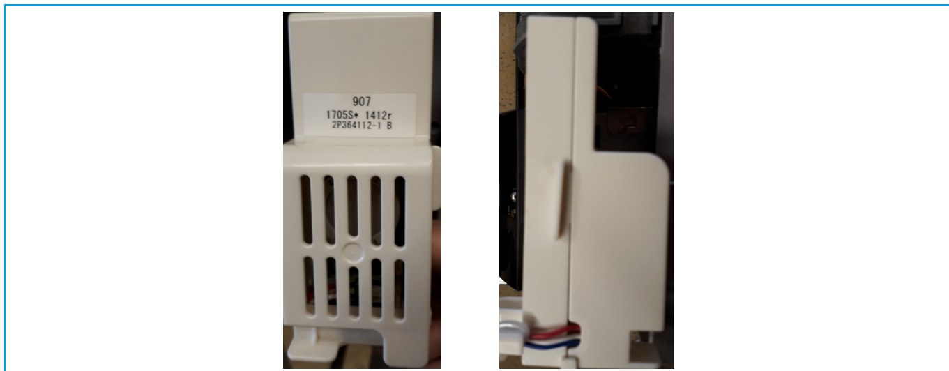
Figure 3-9: Removing casing of the sensor
