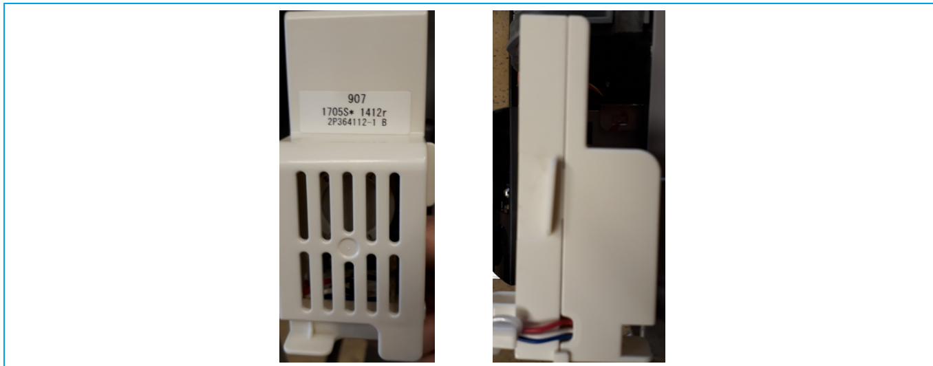
Figure 3-5: Removing casing of the sensor
