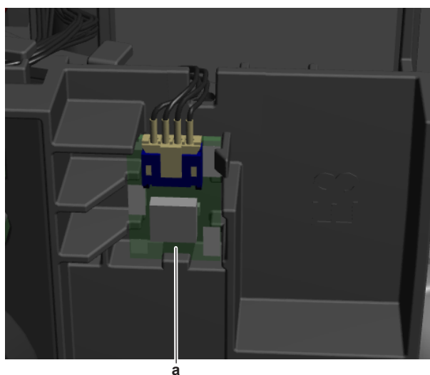
a Humidity sensor PCB assembly
